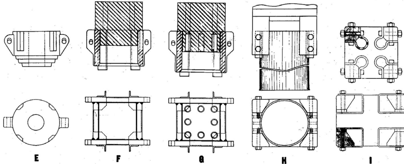
**E**—For driving pipe piles of all sizes. **F**—For driving smooth butt concrete piles. **G**—For driving concrete piles with extended reinforcing rods. **H**—Pipe sleeve, diameter determined by dimension M on page 4. **I**—Filler pieces for various sizes and sections of steel sheet piling or Wakefield wood sheet piling.
