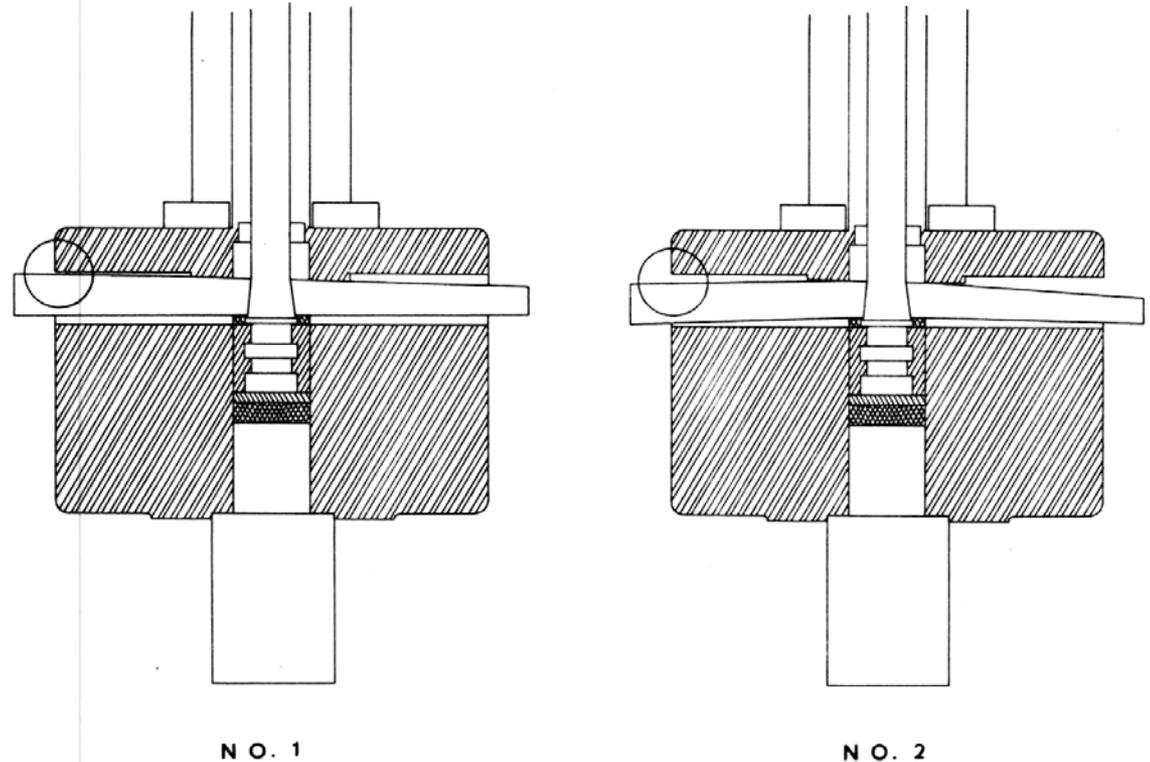
Sometimes it is difficult **not** to tighten the Ram Keys too much. Working with a large sledge hammer a Ram Key can easily be driven so far as to bend. Figure No. 1 shows a Ram Key properly seated. Figure No. 2 shows a Ram Key driven too far and bent. When the Ram Key is first installed there might be a slight gap as circled on drawing No. 1. When driving the Ram Key tight, if the gap starts to widen, as circled on drawing No. 2, then the Key has been driven too far and is bending.
