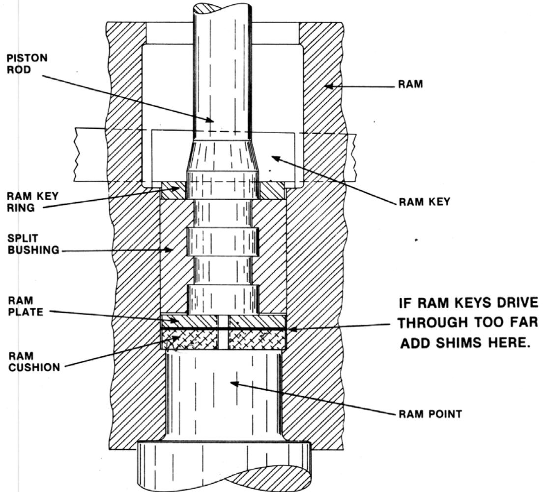
After a Hammer has a lot of "mileage" the parts that hold the Piston Rod to the Ram wear a little. This will necessitate some adjustment to insure proper tension of the Ram Keys. If this condition exists in your Hammer and the Ram Keys have a tendency to drive through too far, add Shims between the Ram Cushion and the Ram Plate.
