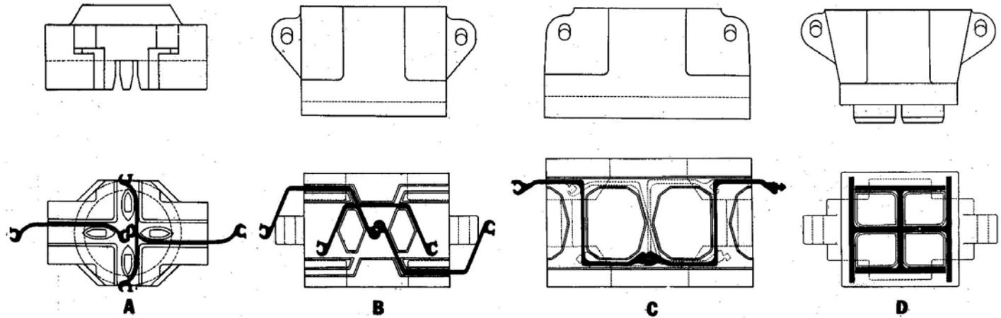
**A**—For driving one and/or two pieces of straight web steel sheet piling. **B**—For driving one and/or two pieces of deep arch steel sheet piling. **C**—For driving one and/or two pieces of Z-section steel piling. **D**—For driving steel H-beam piles.
