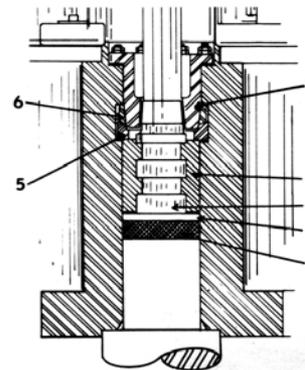
four Dowel Pins, align the Ram Retainer Split Ring (7) around the Piston Rod and insert into Segmental Pressure Ring as shown. Securely fasten all hold-down nuts.
