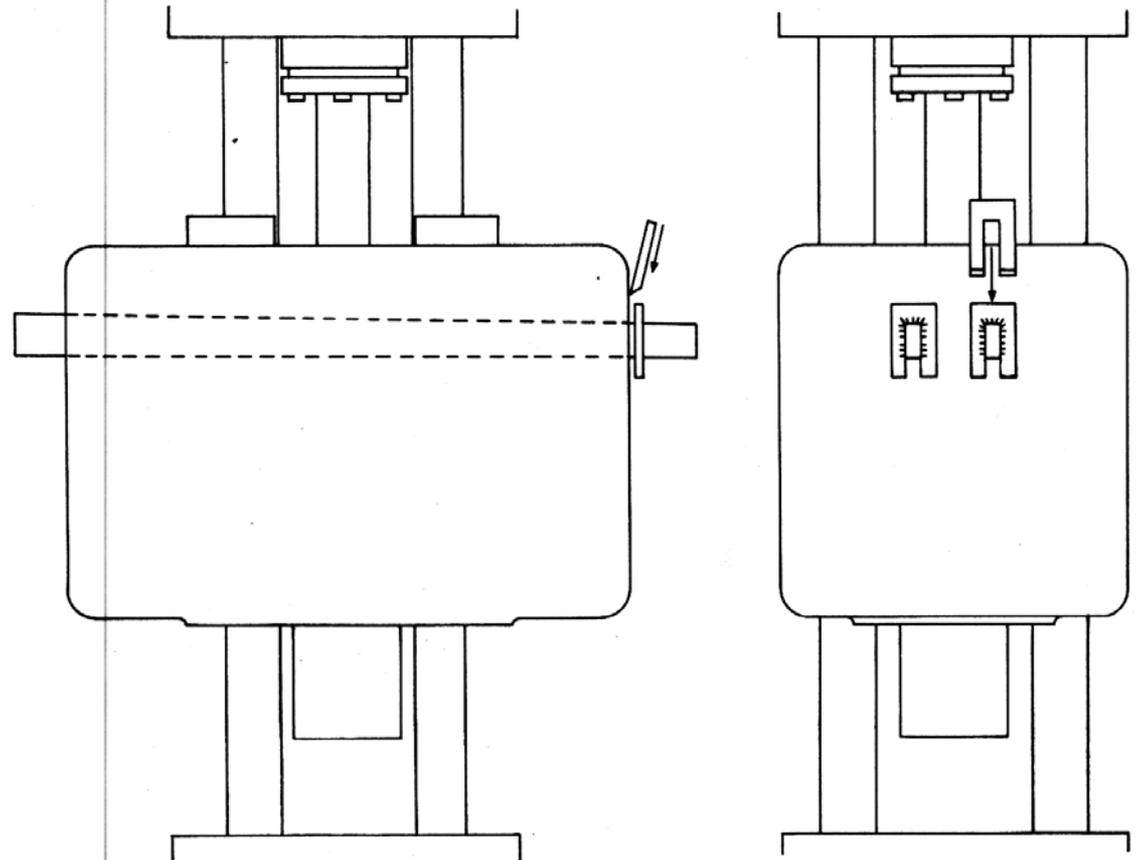
When some hammers get enough mileage on them to warrant retirement and under certain driving conditions, the contractor may have trouble keeping the ram keys tight. Usually under these circumstances, the contractor will weld the keys to the ram and worry about the consequences later. The drawing above shows a better way of keeping the keys tight and allows for quick and easy retightening during the job.
