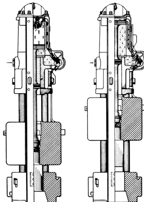
The Differential system requires 1/3 less air or steam as compared to a similar size Double Acting Hammer.
