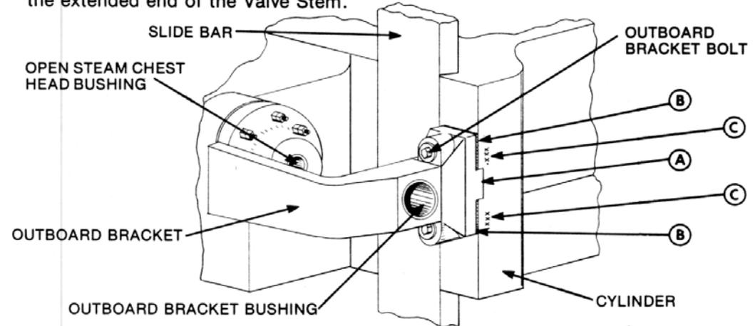
It is absolutely essential in the final installation that the outboard bearing be right in line with the bore of the Bushing in the Open Steam Chest Head. Due to unavoidable differences in the manufacture of the Cylinder and the Outboard Bracket, a certain amount of Selective Assembly is necessary.
