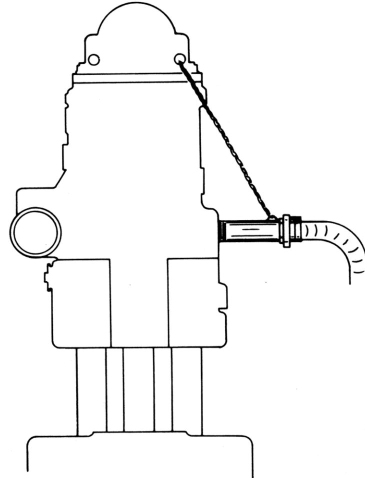
The length of the Nipple from the Inlet must be kept to a minimum. A long Nipple, as shown in the drawing, even though supported by chain or wire rope, will cause damaging leverage and vibration. Extensions to the side, like the arrangement in the picture, allow for good support of the Piping and Hose.
